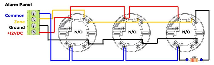
It is important to note that while these smoke detectors are wired together, they do not interconnect. As a result, they do not comply with the NZS 4514:2021 standard as of November 2024.
