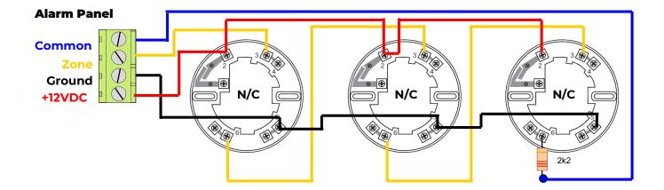
Note: The NB338 smoke detector relay contacts are set to normally open by default. To change the relay state, remove the two screws on the back of the detector and reposition the internal jumper to the "NC" setting. This is illustrated in the manual provided with the NB338.
